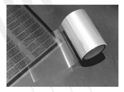
The APF-NS Protection film is a 0.25 mil. (6 microns) thick polyester film developed to protect phototools used in conjunction with liquid solder resists but is also ideal for primary image films. The smooth, non-stick coating prevents particles of photo resist from adhering to the phototool, while minimizing the need for cleaning and inspection. Ideal for track and gap widths down to 0.3 mil (8 microns). The film is completely removable without leaving any adhesive residue.
